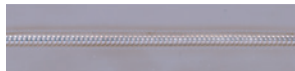
↑ Lap fillet welding (welding w/o rod) of stainless steel(plate thickness: 0.5 mm) (Pulse current: 50 A, Base current: 5 A, Speed: 30 cm/min)
