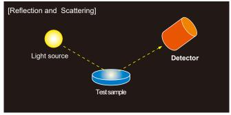
NIR light is commonly used in analytical applications, and halogen lamps are typically selected as the light source. However, as halogen lamps used for general lighting are rapidly being replaced by LED for energy-saving reasons, there is growing interest in alternative light sources for analytical use as well.
