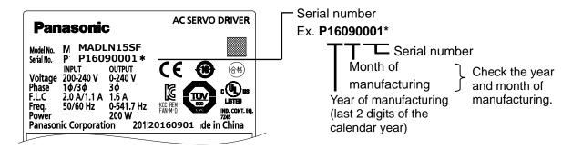
The serial number shown on the label attached to the front surface of the package box follows the following rule.
