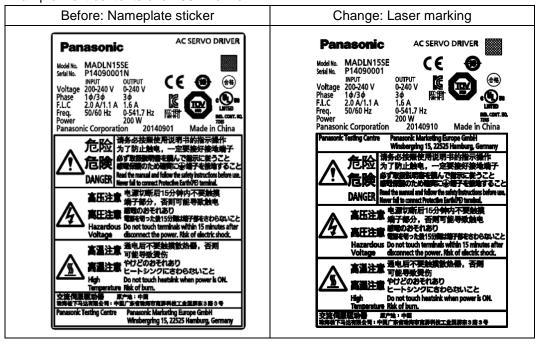
• There is no change to the external dimensions, characteristics or performance of the servo driver due to this specification change.
