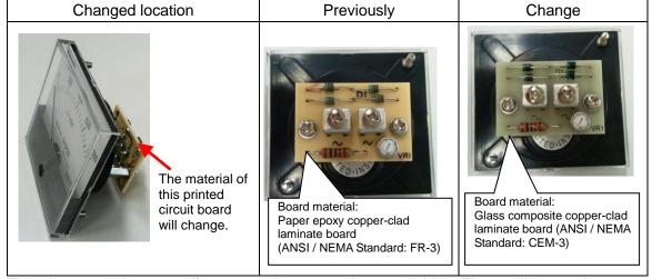
This change will have no effect on product properties or reliability. There will be no changes to the measurements of the printed circuit board.
