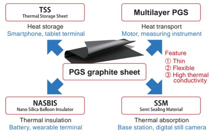
sors will extend the duration of high frequency operations, i.e. duration of crisp and smooth smartphone operations. The SSM, which consists of stacked elastomer and PGS graphite sheet, diffuses heat from its concavo-convex surface. The elastomer layer absorbs heat and the PGS graphite sheet diffuses the absorbed heat. This mechanism serves as thermal management for base stations and digital still cameras. The NASBIS-com-
