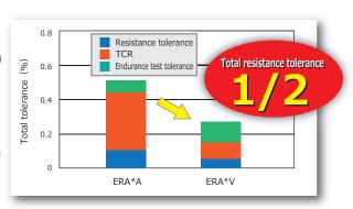
Half total tolerance from thin film chip resistors (Conventional series)
