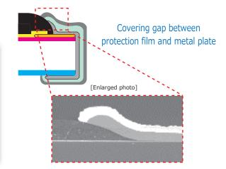
Achieve excellent anti solder joint crack by back side resin layer
