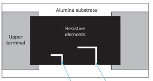
By unique "Double L-shaped trimming" process, we can make slight adjustments of resistance value.
