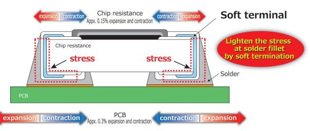
Maintain exellent solder connection reliability even in harsh temperature environment such as for automotive.
