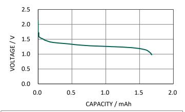
Charging Condition : CV(2.3V, 360 $\Omega$ , 24H, 20°C) Discharging Condition : CR(51k $\Omega$ , 1.0V Cut-off, 20°C)
