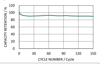
Charging Condition : CV(2.3V, 200 $\Omega$ , 10H, 20°C) Discharging Condition : CR(15k $\Omega$ , 1.0V Cut-off, 20°C)
