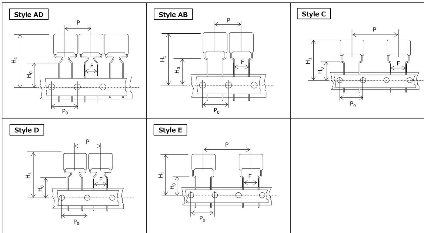
\*: H1 dimension is based on insertion machine "Panaset RH series" made by Panasonic. Consult with Panasonic technical staff when using other insertion machines.
