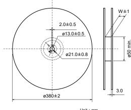
**Taping dimensions** Feeding hole
