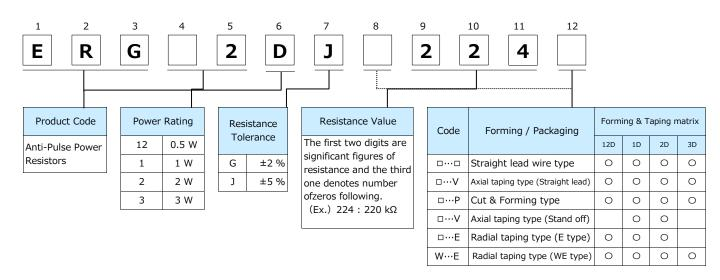
The above example shows an anti-pulse resistor, 2 W power rating, resistance value of 220 k ohms, tolerance ±5 %, and package of standard bulk packing.
