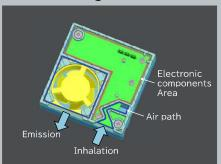
Special inside structure that the air containing fine particles dose not pass upper of PCB, can control performance deterioration.
