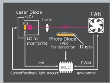
Long life has realized by avoiding unnecessary operation of key parts (Laser, FAN···etc.).
