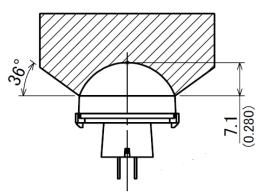
Recommended Hole Drilling Diameter
