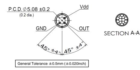
Catalog No. EKMC260181□K Name PIR MOTION SENSOR "PaPIRs" VZ series PaPIRs⁺ model Standard detection type (170µA / Analog output) Rev.
