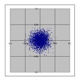
positioning accuracy: 47.2 micron
