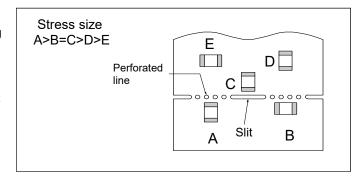
to thermistor placement, consider the board breaking method as well.
