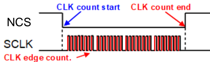
Figure 5-7 SCLK Bit Count Timing
