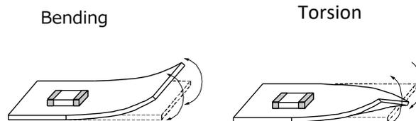
(2) Dividing/Breaking of the PC boards shall be done carefully at moderate speed by using a jig or apparatus to prevent the Inductors on the boards from mechanical damage.
