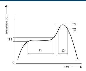
Pb free solder recommended temperature profile Power Choke Coils for Consumer use
