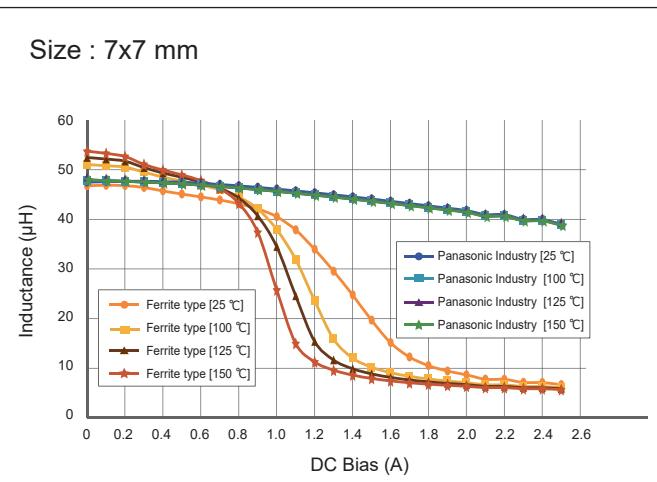
The ETQ-PM Inductor allows for large currents. The inductance levels do not drop significantly as the current increases regardless of the temperature.
