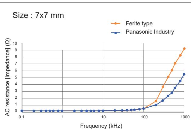
The metal composite molded structure has a distributed gap rather than a discrete gap resulting in low AC resistance (impedance) at higher frequencies.
