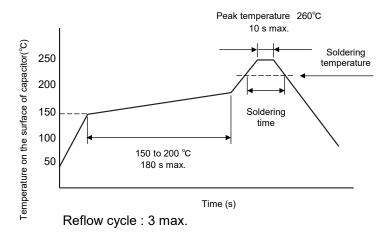
Soldering temperature and soldering time
