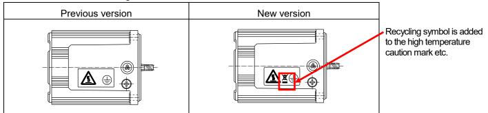
(Drawing indicates 60 mm sq. motor, typical model shown)
