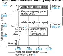
These curves show the characteristics with the maximum sensing range set to 100 mm 3.937 in, 200 mm 7.874 in, each, with white non-glossy paper ( $50 \times 50$  mm  $1.969 \times 1.969$  in).
