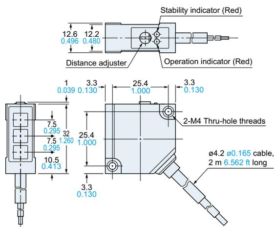
**Assembly dimensions with attached mounting bracket**
