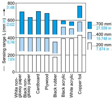
These bars indicate the sensing range with the respective sensing objects when the distance adjuster is set to a sensing range of 700 mm 27.559 in, 400 mm 15.748 in and 200 mm 7.874 in long, respectively, with white non-glossy paper. (Sensing object size: 35 × 60 mm 1.378 × 2.362 in.)
