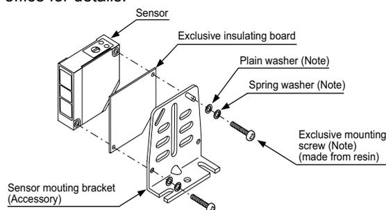
Note: Attached with the exclusive insulating board.
