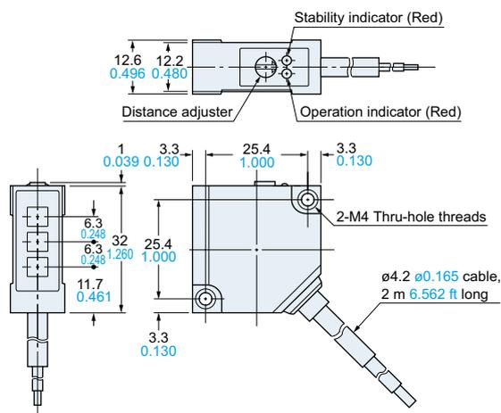
**Assembly dimensions with attached mounting bracket**
