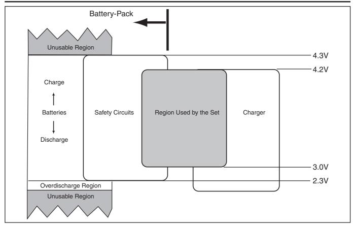
• The safety circuits in the diagram above are for overcharging, overdischarging, and overcurrent for a single cell battery-pack. Please consult Panasonic when two or more cells are connected or when actually using this or other circuits.
