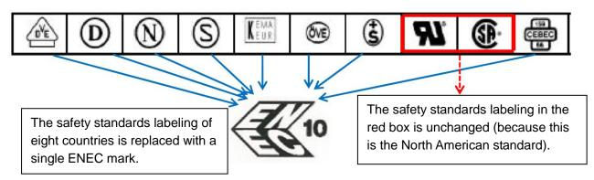
Note: The unified ENEC mark and the North American standard mark are displayed on the reverse of the terminal block and cannot be seen from the outside.
