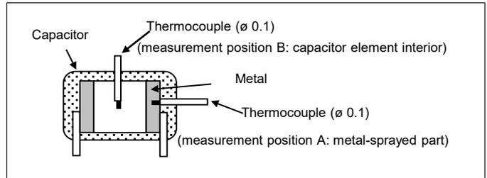
When a capacitor is sent through a high-temperature atmosphere after being subjected to the (flow) soldering process, check the mounting temperature including the temperature of the capacitor in the high-temperature atmosphere.
