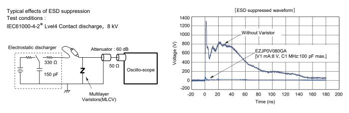
\*IEC61000-4-2 ... International Standard of the ESD testing method (HBM) for electronic equipment ability to withstand ESD generated from a human body. It sets 4 levels of severity
